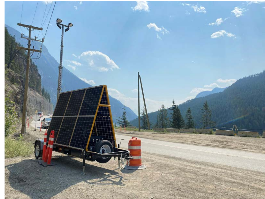
Trialling a solar-powered light tower at the Kicking Horse Canyon – Phase 4 project
